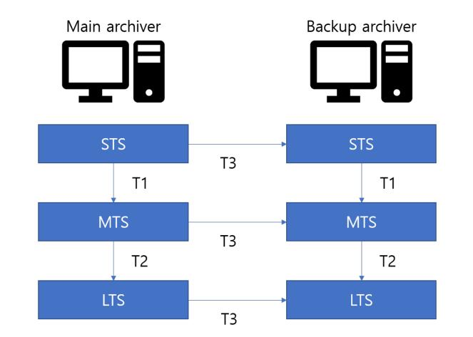
STS uses SSD MTS and LTS uses HDD
