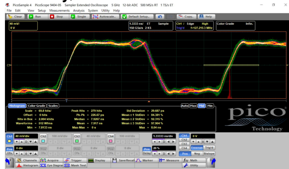
No delay, crosstalk around the clock edge
