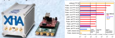
Figure 1. Summary of FWHM time resolution for various signal sources and PTP/SyncE network configurations with Pixie-Net electronics (pictured left)
