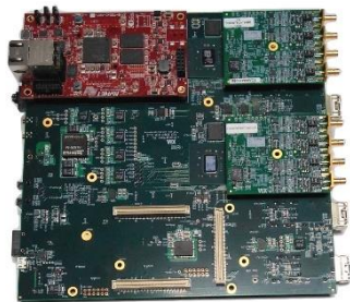
PXdesk main board with ADC daughtercards and Zynq controller
