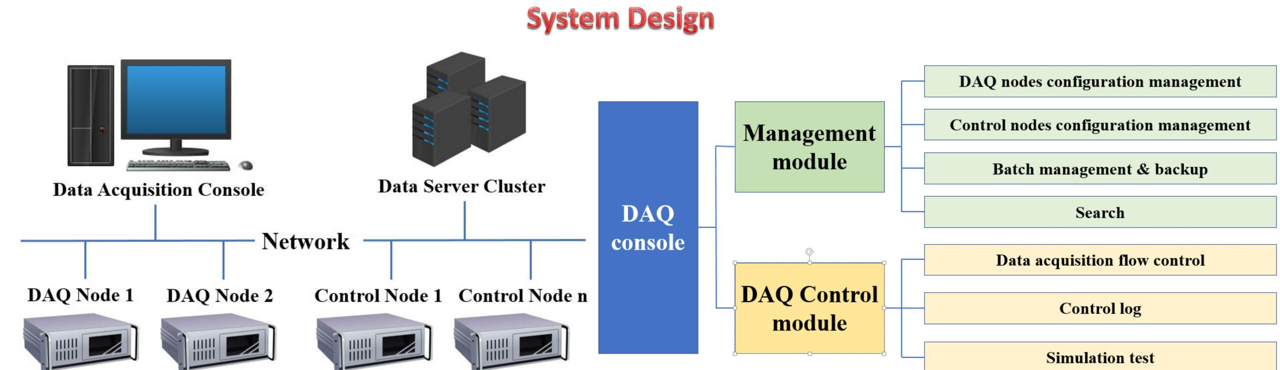
The EAST data acquisition system includes a data acquisition console, data server cluster, DAQ nodes, and control nodes. All the components are in a local area network (LAN). The improvement is about the data acquisition console (DAQ console). The DAQ console is divided into 2 modules: management module and control module.
