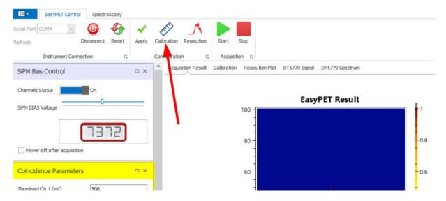
The EasyPET will perform two rotations to reference its position. Be careful that the signal and trigger cables do not obstruct this movement. Once stopped the GUI will show the number of coincidence counts from both detectors.
