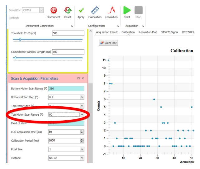
Start the acquisition. It will take around 40 minutes to complete a scan. You will slowly see the PET image being built up in the GUI
