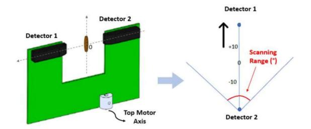
In order to understand this movement run it once with a very limited scan range for the top motor. In the EasyPET tab, go to "Scan & Acquisition Parameters" and change the "Top Motor Scan Range" from 90 to 0.9
