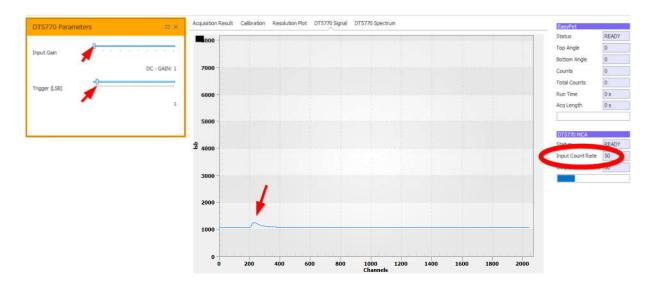
Observe how the rate goes up when you bring the source close to the detector (the rate is shown in the GUI and also on the MCA display).
