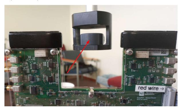
The first task is to make sure that the source is really in the detector center. This operation is somewhat difficult because the source and the detectors are both really small, and it is quite hard to properly align them.
