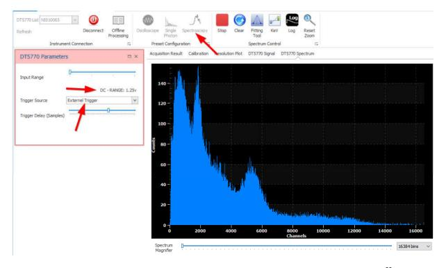
Observe the Compton spectrum and the 511 keV peak. Can you see 1275 keV from the Ne<sup>22</sup> decay? Use the fitting tool to check the position of the two peaks.
