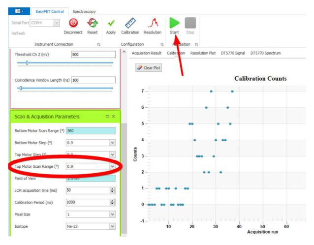
Run the acquisition and observe the two motors' motion. Observe how the source always stays between the two detectors. In the end the bottom motor goes back to the starting position. (Don't worry about the acquired image; that will come in the next step).
