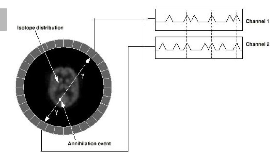
• LOR (lines of response) arranged into sets of 1-dimensional parallel projections
