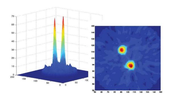
$^{22}\text{Na}$  sources, 5  $\mu\text{Ci},$  2.7 mm Ø and 9 mm apart.
