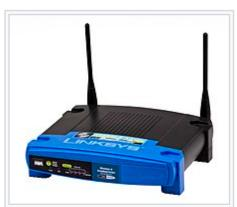
This Linksys WRT54GS WiFi router from 2005 operates on the 2.4 GHz "G" standard, capable of transmitting 54 megabits per second.
