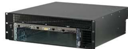
6U 6 Slots Right-to-left cooling 450W/slot
