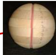
Tumour with insert for dose measurements with film
