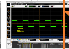
Fig.10. Generated AO period(10kHz, 100usec)
