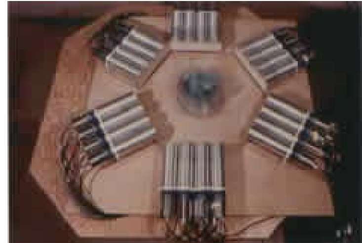
1973-74: "PETT II" hexagonal array, 24 NaI(Tl) detectors, Ter-Pogossian et al., Washington University, St.Louis.
