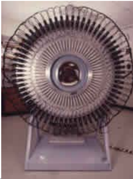
1973: "Positome I", first circular ring PET scanner, 32 NaI(Tl) detectors. Built at BNL and used for blood flow studies with ^{77}\text{Kr} . Transferred to Montreal Neurological Institute in 1975.
