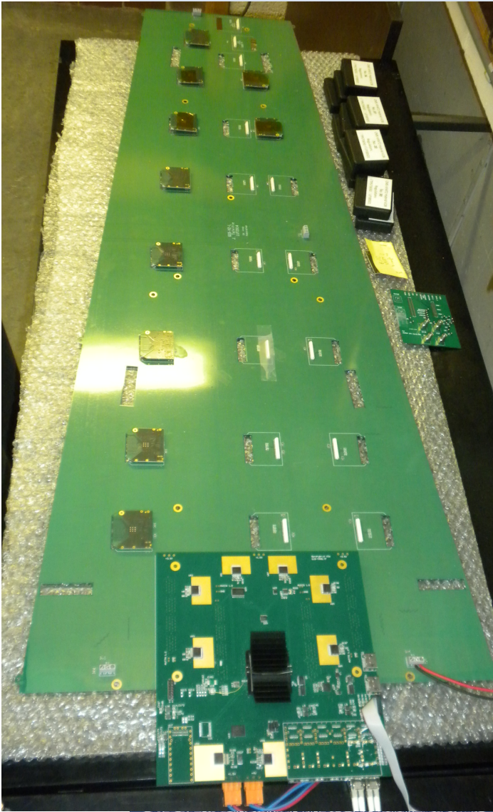
Photograph showing the GEM readout system for the upgrade of the CMS forward muon spectrometer. The system is designed to improve the trigger efficiency of the CSC system.
