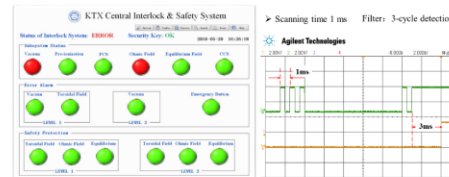
Fig. 6. Touch panel of Interlock & Safety system
