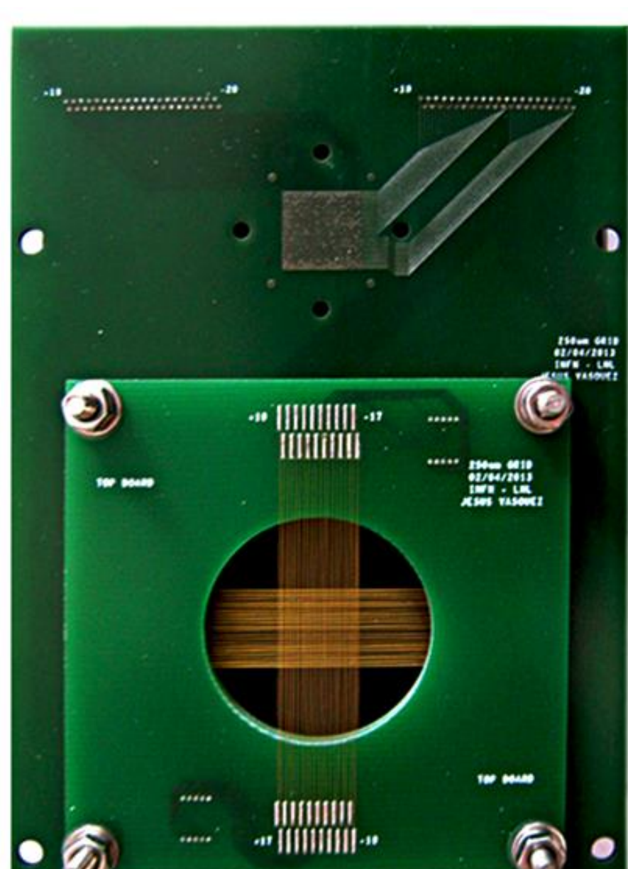
Beam Profiler Monitor (BPM)
