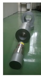
Figure 2. SPEC: (from the top) Lead shield, Anti Compton Shield, CeBr3 detector.
