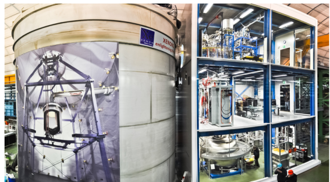
Fig. 1. The Xenon1T underground facility at Laboratori Nazionali del Gran Sasso (LNGS), in Italy. At the left the water tank that holds the TPC inside and on the right the support 3 plan building.
