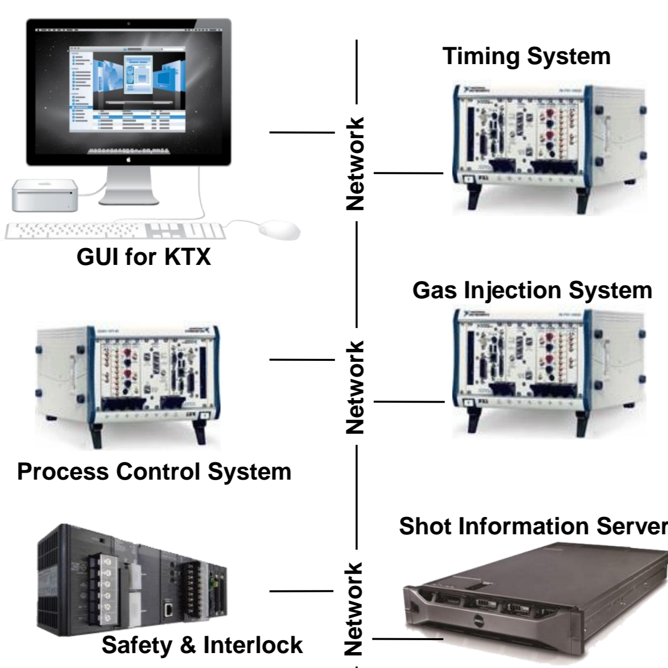
Fig. 2. Structure of KTX central control system
