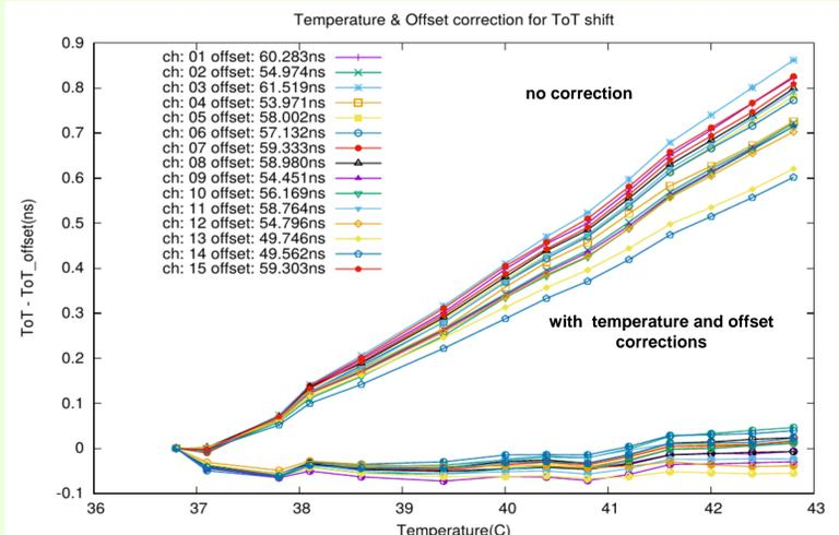
Time over Threshold (TOT) values measured with the FPGA TDC are also affected by temperature. Both the fine time counter calibration and the stretcher offset for the trailing edge signal are temperature dependent. This deterioration of ~100 ps/°C can be compensated by individual channel calibration with a pulser signal of known TOT. Such correction can be applied in stream/DABC software already during data taking, since the actual temperature data is also read out from the FPGA. Taken from [1]
