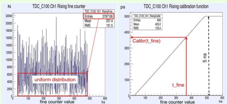
accumulated fine time counter distribution of a single TDC channel
