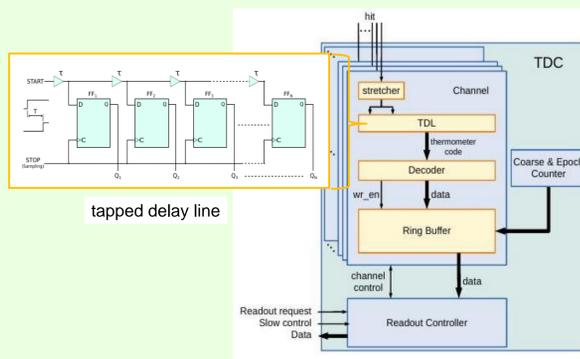
TRB3 FPGA TDC uses tapped delay line (TDL) technique: Fine time stamp of an incoming signal is derived from the number of delay elements which the signal propagates from arrival until the next 200 MHz readout clock edge stops such sampling. For time over threshold (ToT) measurements, trailing edge is shifted by a stretcher to subsequent readout clock cycles (from [1]).
