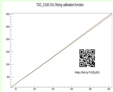
Figure shows the calibration function for the same channel, measured with temperatures 28, 35 and 44 °C. These calibrations look very similar except for a scaling factor. This can be described by a linear function:
