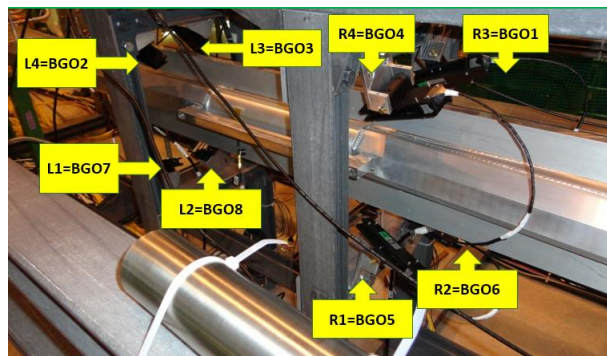
Fig. 2. The installation of 8 BGO crystals around the interaction point. The R1-R4 crystals are at the +z side and the other 4 the -z side. In the Belle II coordinate system, the +z is close to the direction of the electron beam.
