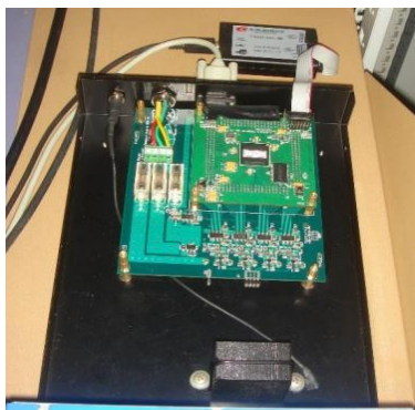
Fig. 4. The inside of BGO DAQ system box. Near the bottom of this picture is the MAMPT. The FPGA board is plugged on top of the main DAQ board.
