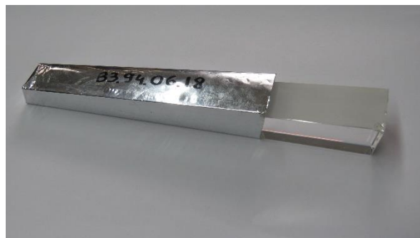
Fig. 1. The BGO crystal in our beam background monitoring system. In the figure, the crystal is half-pulled out from the wrapping material for demonstration purpose.
