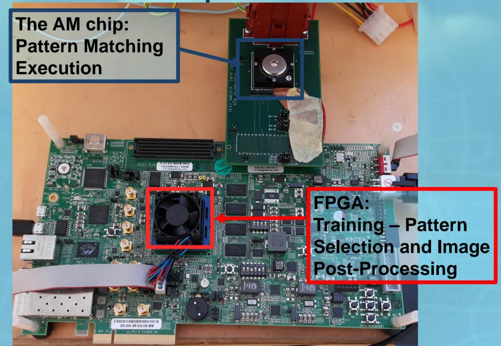
The simplest hardware system we can use is a combination of a Xilinx Kintex Utrascale evaluation board (KCU105) with a small mezzanine card housing the Associative Memory chip AM05, both designed by M. Beretta, F. Crescioli, A. Stabile et. al [3].
