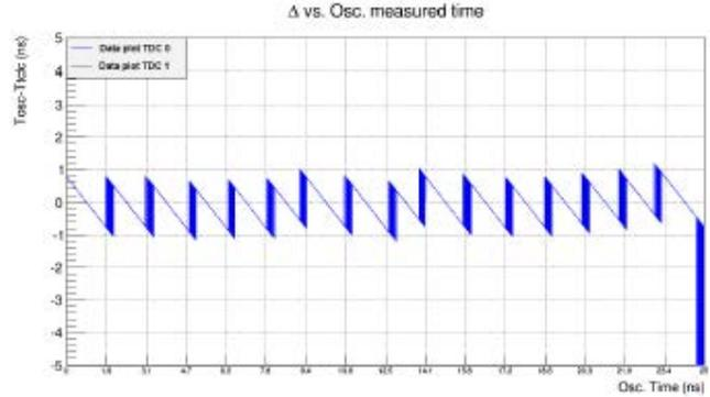
Fig. 6. Difference between TDC and scope measurements
