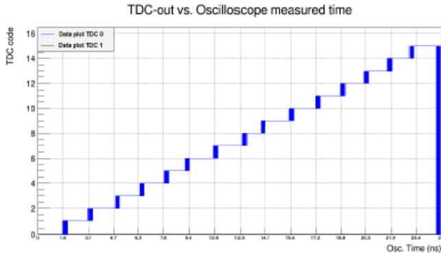
Fig. 5. Phase measured by scope versus TDC output code.
