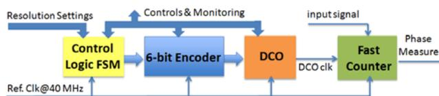
Fig. 2. Simplified block diagram of the TDC.
