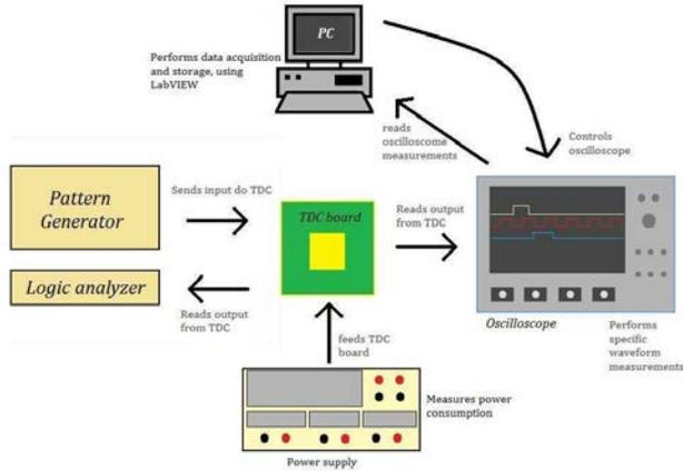
Fig. 4. Scheme of the setup for the ADV2 chip test.
