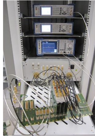
Figure 4. Automated test stand for RTM Backplane RF performance tests.
