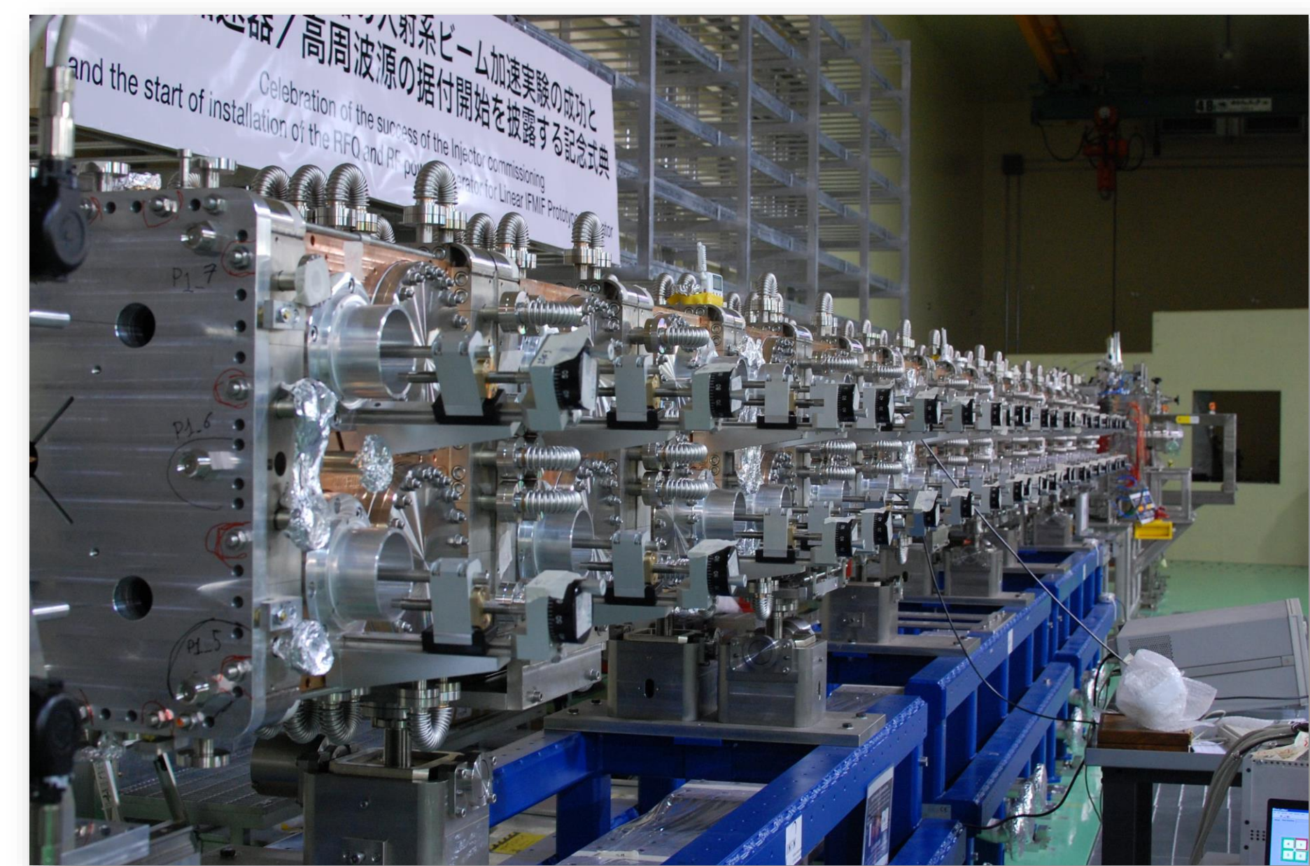
Figure 5: RFQ Installation in Rokkasho
