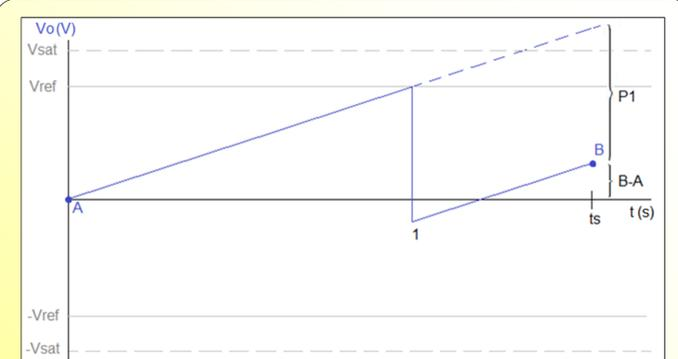
The plot shows the integrator output voltage for negative constant input current. The dashed line represents the output front-end voltage without CPS, which results in saturation for a given input current. By injecting the negative charge pulse (P1), saturation is avoided, thus extending the dynamic range of the input current.
