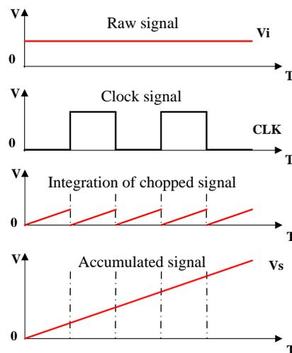
Fig. 3. Principle of the chopper.
