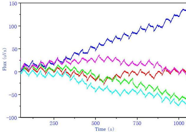
Fig. 7. Integration drifts of 1000 s when the input is shorted.
