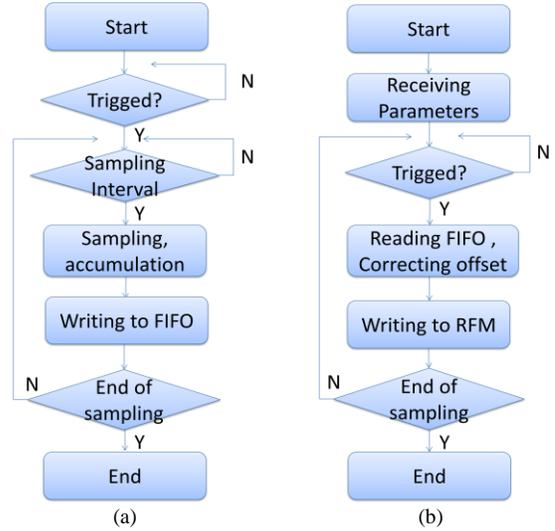
Fig. 5. Program flow chart of the hybrid integrator. (a) Program on FPGA, (b) Program on LabVIEW RT.
