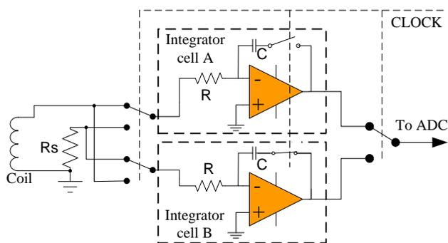
Fig. 2. Schematic of the integrator chopper.
