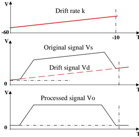
Fig. 4. Algorithm of linear drift compensation.
