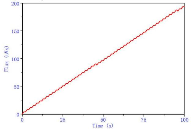
Fig. 6. 100 s integration when the input is connected to a 2 mV source.
