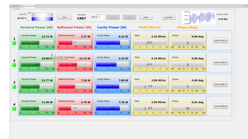
Figure 3: CSS Interface for monitoring the working status of a cryostat.
