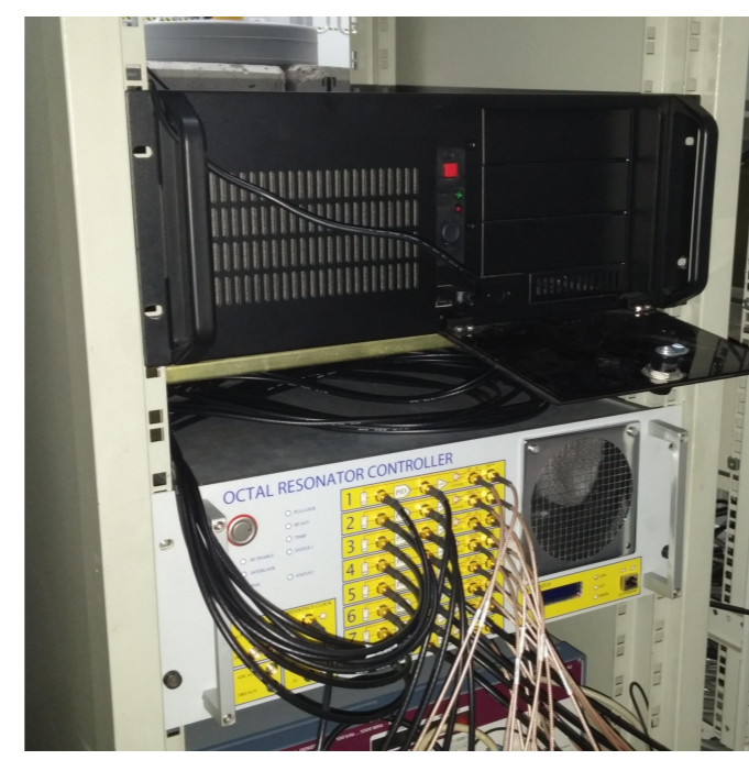
Figure 2: Setup used for field test of the new RF control system. The rack contains a personal computer (PC) and the octal resonator controller (OCR).
