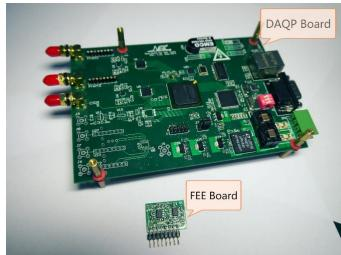
Fig. 3. Prototype print circuit board (PCB) of the DAQP Board and one FEE Board.
