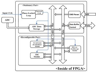
Fig. 4. FPGA internal logic block diagram
