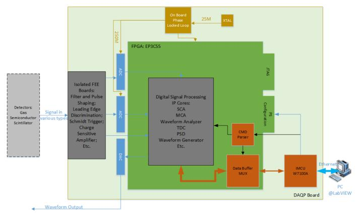
Fig. 2. Schematic Block diagram of the DAQP System. The DAQP system mainly consists of four parts: FEE Boards, DAQP module, Reconfiguration module and PC Software. In a specified experiment, appropriate FEE Board will be plugged into the socket on DAQP Board, and Reconfiguration module along with PC Software will decide which digital processing IP core to use. The four parts work together to realize remote data acquisition and real-time data processing for various experiment applications.
