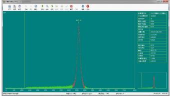
Fig. 7 Alpha energy spectrum of <sup>239</sup>Pu
