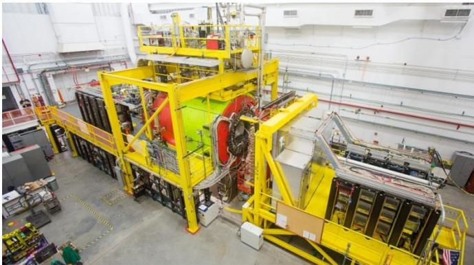
9 GeV tagged polarized photons and a  $4\pi$  hermetic detector
