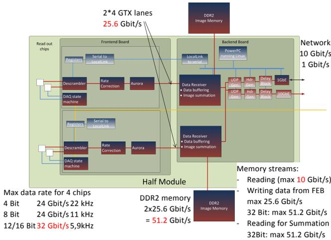
Fig. 5. Showing the maximum data rates at several points. It also shows the bottlenecks which are the memory in 32 bit mode and GTX transceivers in 16 bit mode as well as the 10 Gbit/s Ethernet.
