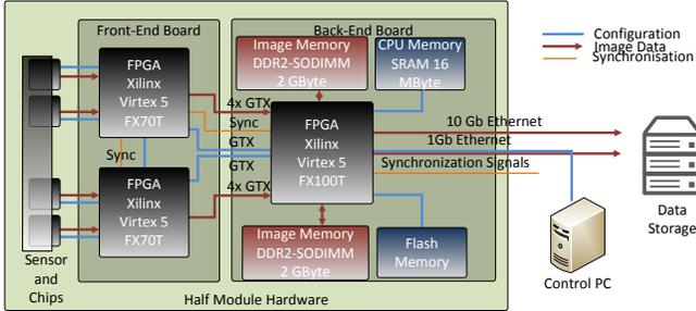
Fig. 2. EIGER half module with sensor, readout chips, front-end, and back-end board.
