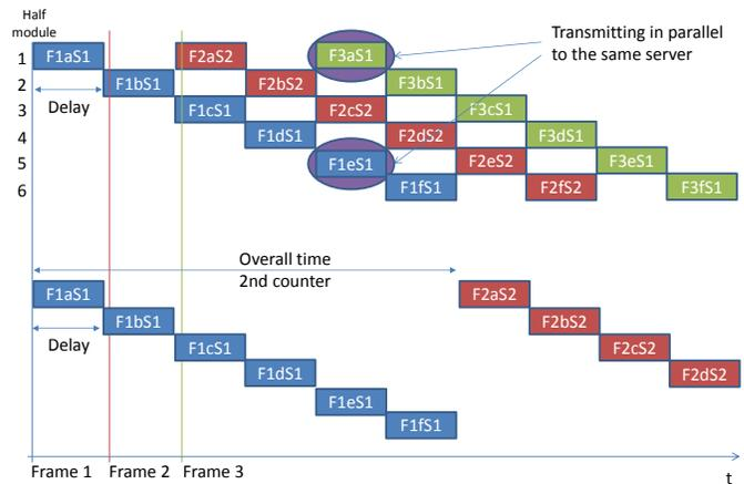
Fig. 7. Round Robin and Delay with two servers. In the upper part the possible conflict of sending to frames to a server at the same time (here F3aS1 and F1eS1) is shown. (F1aS1 means Frame 1 Part a send to Server 1)
