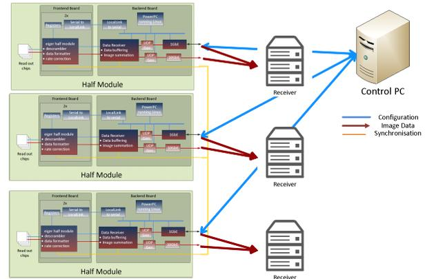
Fig. 6. Network configuration of the EIGER detector. Each half modules is connected to the control PC and to one receiver each.
