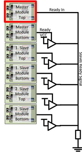
Fig. 3. Ready signal pulled up by the slaves when not ready and released otherwise. Method is proved to work for at least the 2 Mpixel detector with its 8 half modules.
