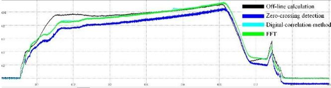
Fig. 3. The comparison of phase shift calculation algorithms. The real-time FFT is in good agreement with the off-line calculation.
