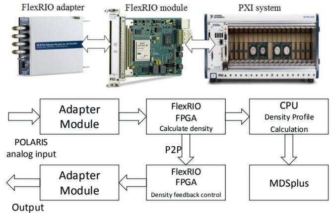
Fig. 2. The structure of POLARIS data acquisition system. The real-time density calculation and feedback control algorithm are implemented based on the FlexRIO FPGA.
