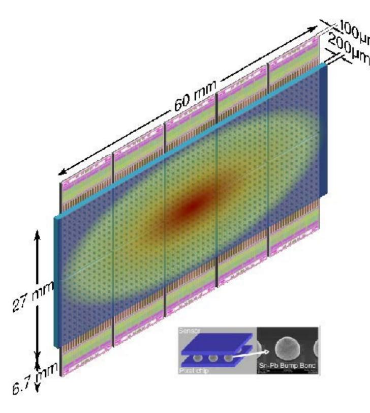
Sensor [FBK,CIS] Both p-in-n/n-in-p Bias: 300 - 600 V Thickness: 200 µm MPV Charge per MIP: 2.4 fC
