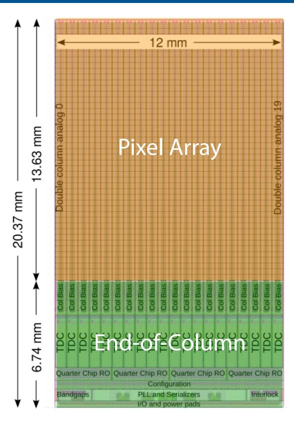
Design by Cern PH-EFE: -1800 pixels (40col × 45pix) -each pixel (300 × 300) µm<sup>2</sup> -separate analog-digital: no high freq clock to pixels
