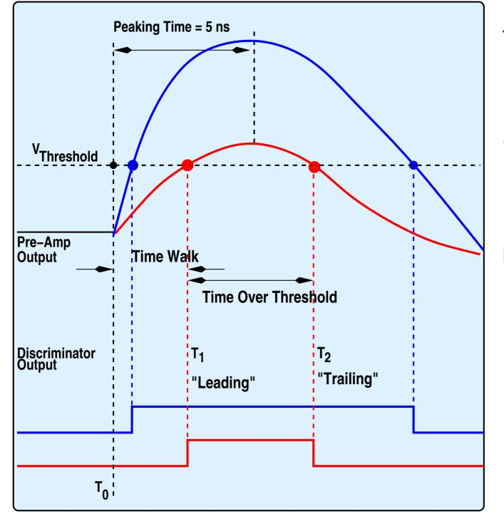
Time walk correction takes advantage of the relation between time walk and time-over-threshold.
