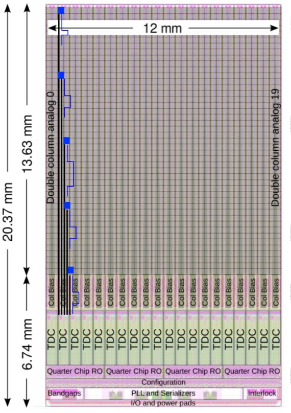
Signals from 5 non adjacent pixels in a column are sent to a multiplexer (HitArbiter)
