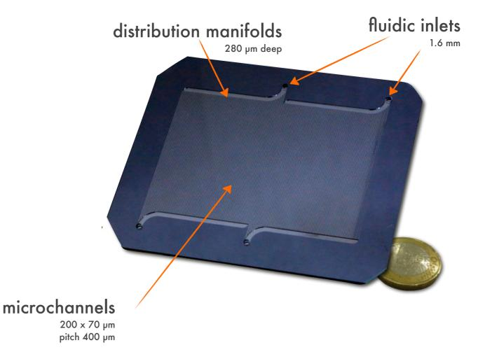
▶Detector glued on 130 µm Silicon Cooling Plate
