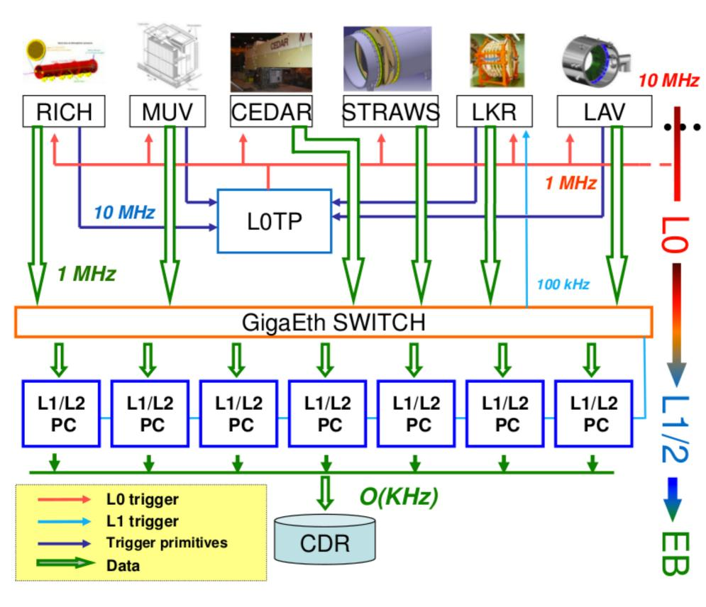
LO: hw synchronous level. 10 MHz to 1 MHz
