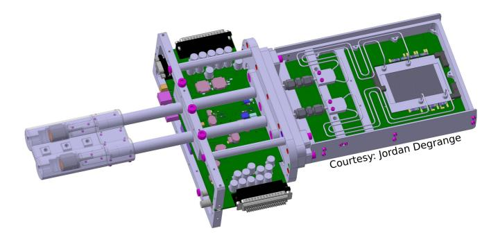
Detector glued on 130 µm Silicon Cooling Plate
