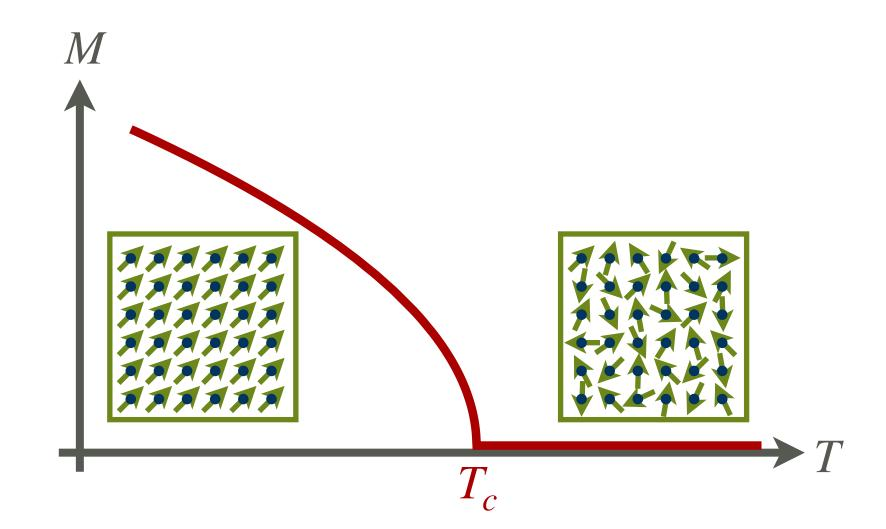
Common examples: ferromagnetism, superconductivity, crystals, ...
