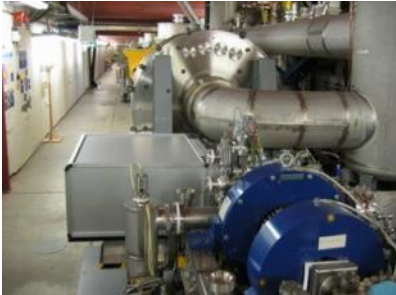
> Normal conducting 1.3 GHz RF gun > Ce 2 Te cathode > Three photocathode lasers
