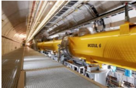
> TESLA type superconducting accelerating modules 1.3 GHz
