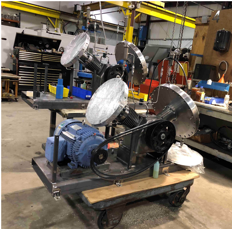
Circulation Compressors under construction (2 of 4)
