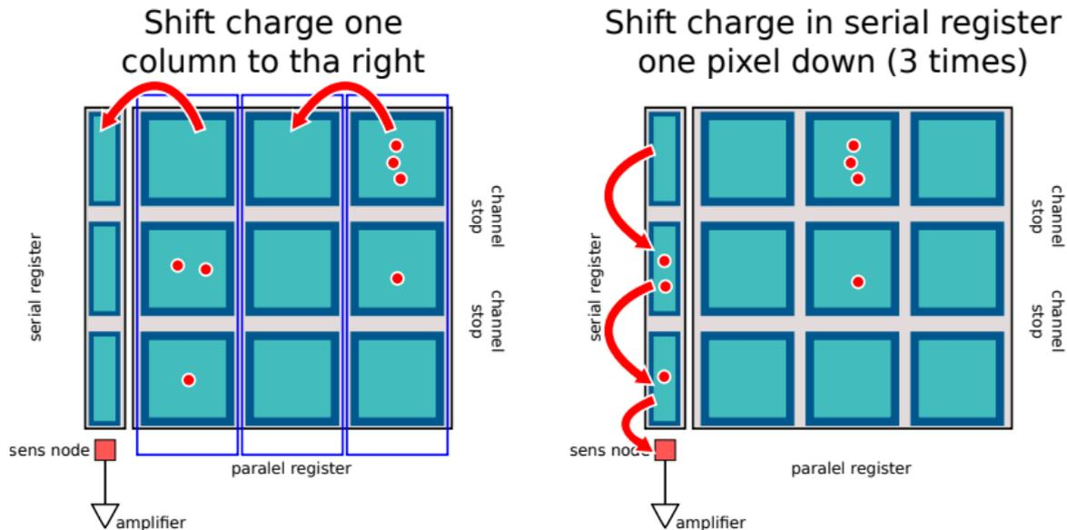
capacitance of the system is set by the SN:  $C=0.05\text{pF} \rightarrow 3\mu\text{V}/e$
