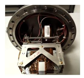
Silicon 3D pixels placed in 2 stations at 210m and 220m from the interaction point measure the deflection of the protons surviving the collision
