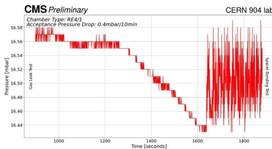
**Figure 4** - This plot shows the gas leak tightness and spacer bonding test for an iRPC gap at CERN. The gas leak test indicated a decrease of 0.15 mbar/10 min, well below the 0.4 mbar/10 min limit. The spacer bonding test showed smooth transitions, confirming good bonding quality. Overall, the detector met the required standards, allowing progression to the next quality control stage.
