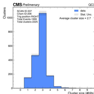
**Figure 5** - The plot shows the cluster size distribution at a working voltage of 7.05 kV for an iRPC detector. Cluster size, which represents the number of consecutive strips activated by a muon, varies due to strip widths ranging 0.60 - 1.23 cm, with strips around the scintillators measuring about 1 cm. This variation impacts spatial resolution. The data was collected with cosmic muons.
