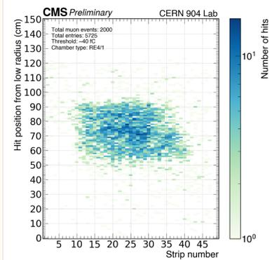
**Figure 6** – Upper: The plot shows a 3D reconstruction of muon hit positions for an iRPC chamber at a working point with a charge threshold of 40 fC. The data was collected using a triple scintillator coincidence trigger with area of 30x40  $cm^2$ .
