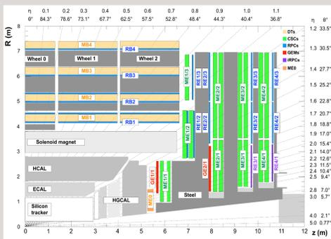
**Figure 1** - A quadrant of the CMS experiment. In purple, the locations of the two endcap iRPC stations - RE3/1 and RE4/1.
