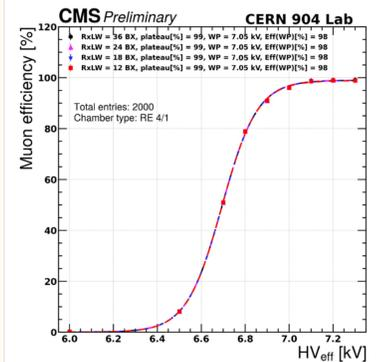
Lower: The plot displays cosmic muon detection efficiency versus effective high voltage (HVeFF). Efficiency peaks at 99%, with the working point defined as the voltage at which efficiency is 95% (HVknee) plus 150V.
