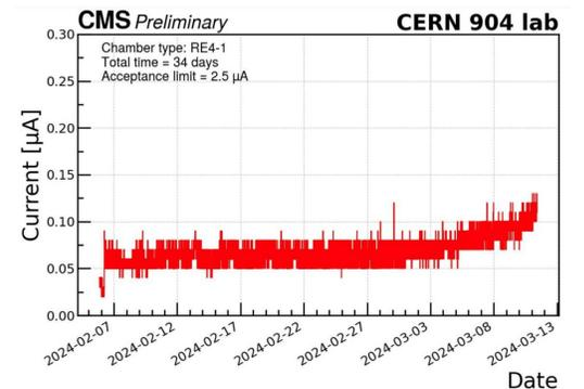
**Figure 7** - Plot illustrating the long-term stability validation test for the chamber. The graph shows the current of one of the two high-voltage layers of an iRPC production chamber maintained at 7kV over a period of more than a month. The current acceptance limit for a chamber to pass this test is 2.5  $\mu A$ .
