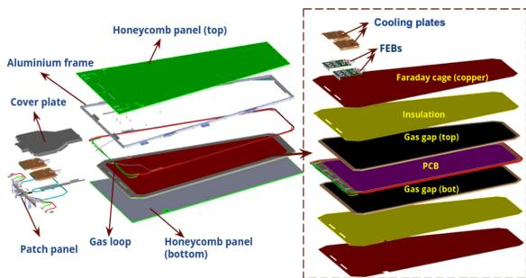
**Figure 2** - Illustrations of the internal structure of an iRPC detector. The detector consists of multiple layers, including two mylar sheets on top and bottom for insulation, two gaps and two printed circuit boards (PCB), all enclosed within a Faraday cage. The HV is high voltage, and FEB is Front-End-Board.
