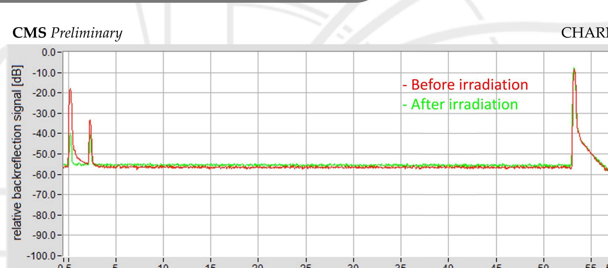
The data obtained with the OTDR (optical time domain reflectometer) show no significant attenuation effect on the optical fiber after the CHARM irradiation period, corresponding to 147 Gy of received dose. Based on this result, these fibers meet the total integrated dose requirements equivalent to ten years of HL-LHC operation, 10-12 Gy, with a safety factor close to 15.
