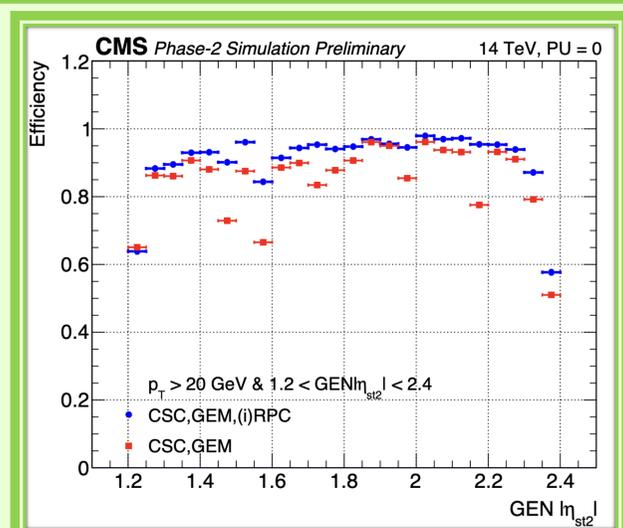
Efficiencies demonstrating the contribution to the EMTF++ algorithm of both RPC and iRPC; these plots show how inefficiencies due to geometry of the other subsystems are recovered by the addition of (i)RPC. The algorithm at this stage is not optimized to account for the absence of subdetector systems.
