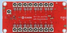
**A5256** — 16+1 channel single threshold, 8+1 channel dual threshold edge discriminator adapter
