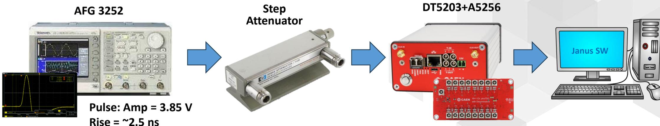
**Common Start Acquisition:** start on Ch0 with fixed amplitude, stop on Ch1 and Ch2 (dual threshold) with variable amplitude (max = 3.85 V). Delay = 13 ns
