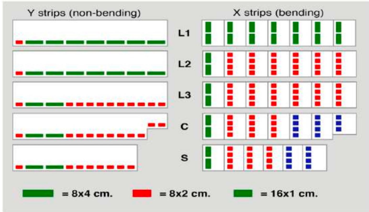
Scheme of the layout of the front-end electronics with different strips pitches
