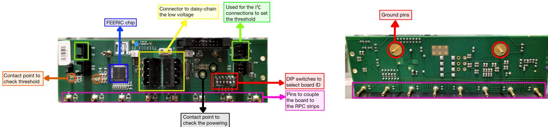
**FEERIC (Front End Electronics Rapid Integrated Circuit), signal discriminator, new Run 3 electronics**
