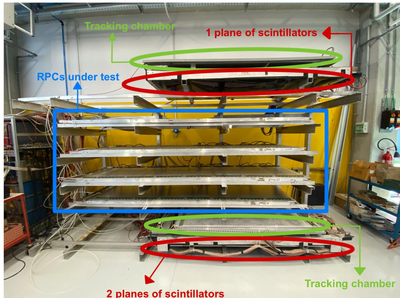
Torino laboratory test setup
