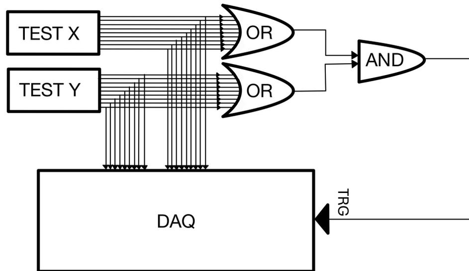
Circuit scheme for dark rate measurements
