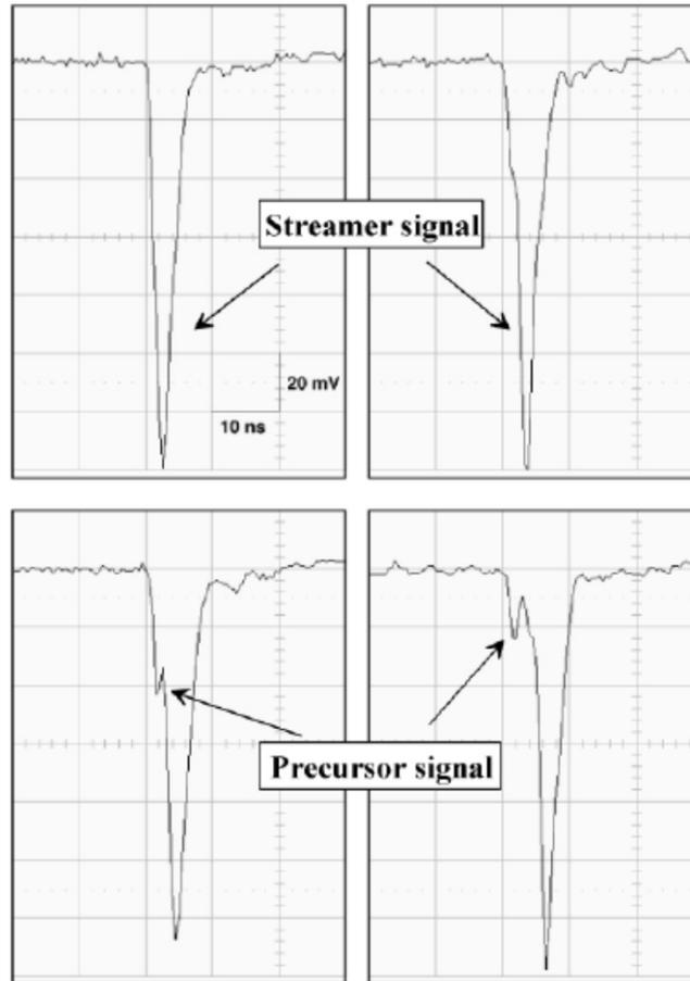
The **streamer** signal has a typical amplitude of **hundreds of mV**, while the **avalanche** one of **few mV**.
