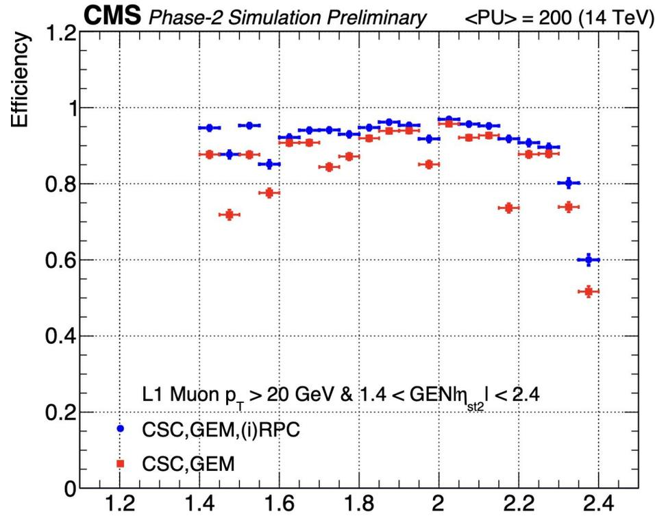
Different values of the EMTF efficiency with (blue) and without (red) the (i)RPC information added to the algorithm.
