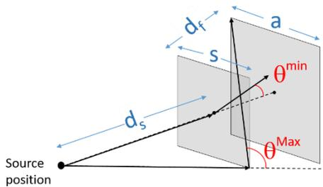
$$\delta\theta = \frac{E}{\sin\theta} \sqrt{\left(\frac{1}{E'^2} \left(\frac{\delta E'}{E'}\right)^2 + 2\sin^2\theta \left(\frac{\delta r}{r_{12}}\right)^2\right)}$$
