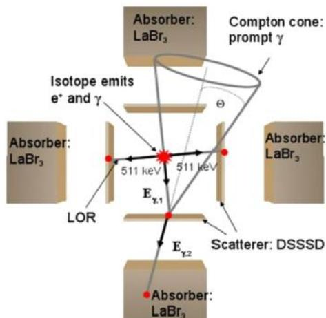
Fig. 3. Schematic illustration of the gamma-PET technique based on multiple Compton arms proposed in [58], which could be extended to hybrid operation by
