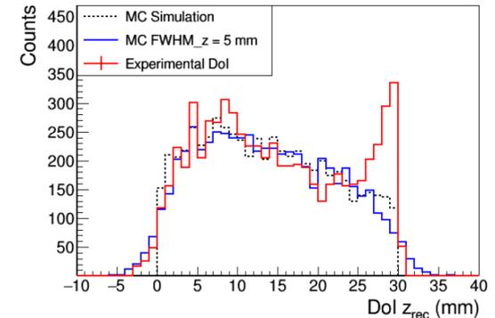
The measured values for  $A_w$  at half maximum (already calibrated) are compared against MC calculated DOIs and true or ideal simulated DOI values.
