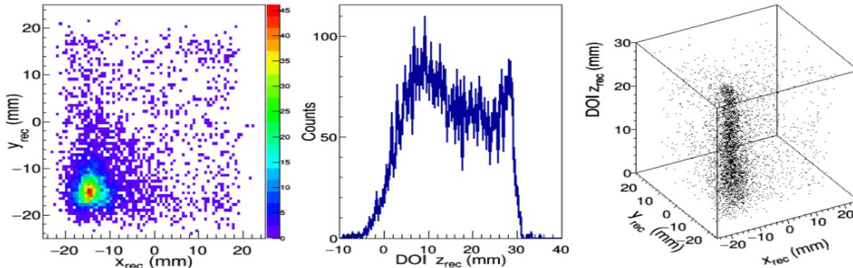
reconstructed DOI coordinates for a peripheral scan position
