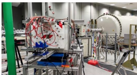
miniBELEN: modular neutron counter for ( \alpha ,n) reactions
