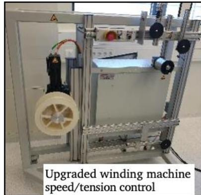
Upgraded winding machine speed/tension control
