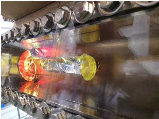
The target cell made of Mylar
