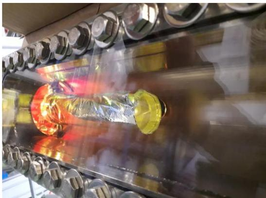
The target cell made of Mylar
