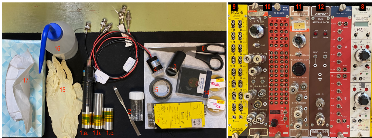
Figure 4. Scintillators and materials needed for this experiment.
