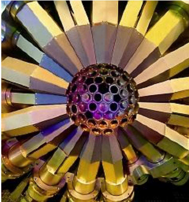
up to 110 Compton-Suppressed Ge detectors
