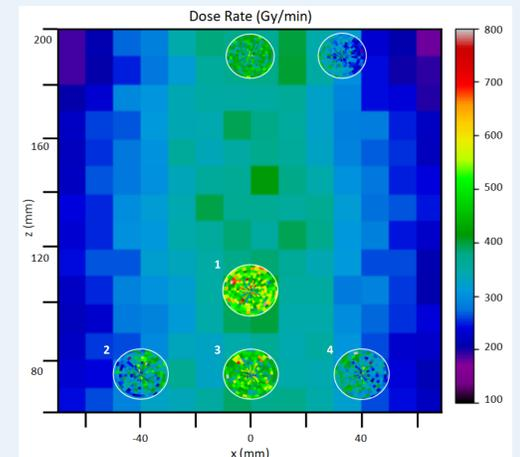
**Figure 3:** A scale representation of the simulated dose rate 7mm from the sources during irradiation of the UTs at the Dalton Cumbrian Facility Co-60 irradiator. The probes are outlined in white. There is a strong directional component to the magnitude of the dose rate. 61.5 million Co-60 decays.
