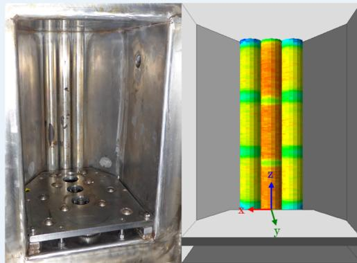
**Figure 1:** Photograph of the DCF Co-60 irradiator and the geometry of the simulation with the photon flux exiting the source guide tubes overlaid
