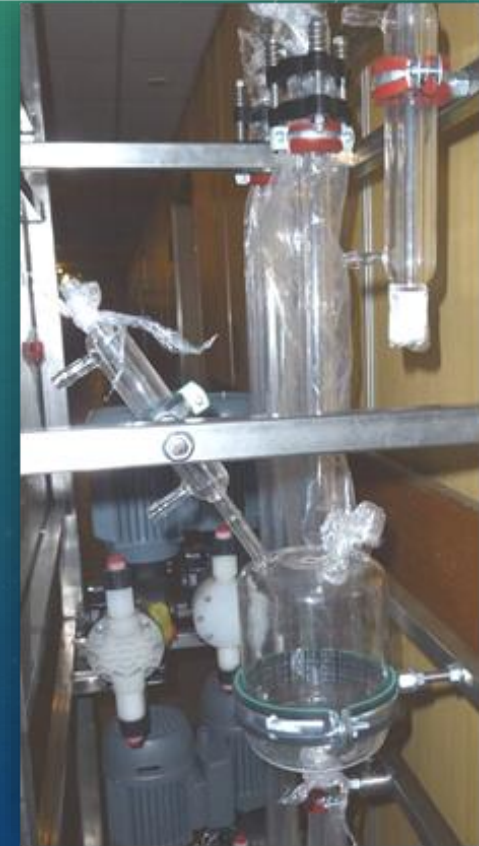
Fig. 1. Diagram and photo of the rectification unit of the setup for purification of the isotopic \text{GeCl}_4 . 1 — central tank; 2 — column for removing of high-boiling impurities; 3 — column for removing of low-boiling impurities; 4, 5 — coolers; 6, 7 — boilers.
